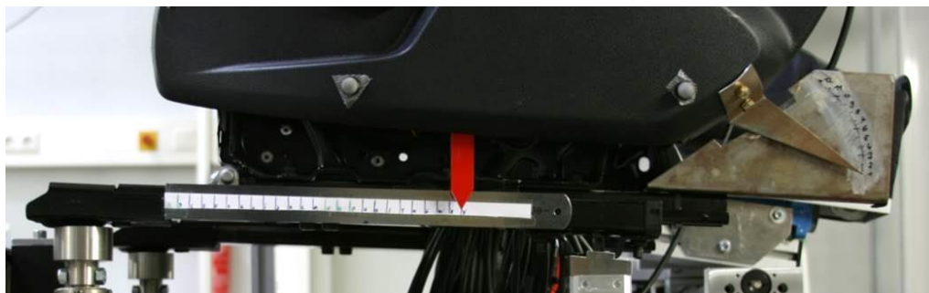
Figure 5.2: ErgoBuck seat adjustment scale for longitudinal and vertical direction.
