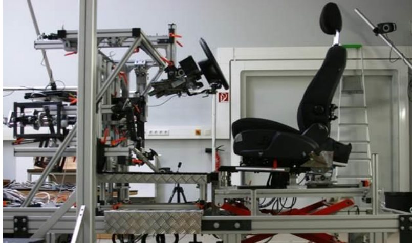
Figure 5.1: ErgoBuck adjusted to the test vehicle main package dimensions.
