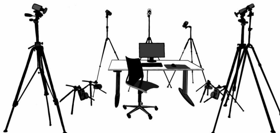
Fig. 2 Standardized testing station with 10 motion capture cameras
