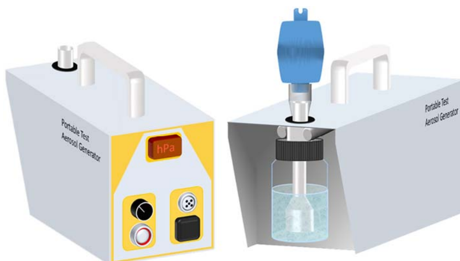
Figure 2.1 Schematic illustration of the aerosol test generator (model 3073 by TSI)
